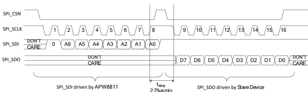
Figure 15. Three/Two-wire SPI Read Operation
