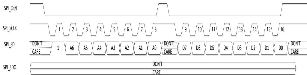
Figure 13. Three/Two-wire SPI Write Operation
