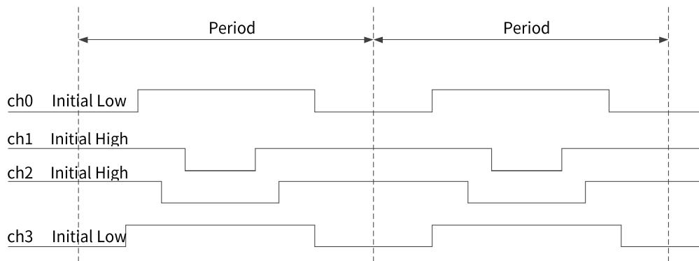
Figure 24. Edge-aligned PWM
