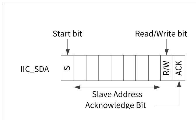
Figure 6.I<sup>2</sup>C Byte Write Format
