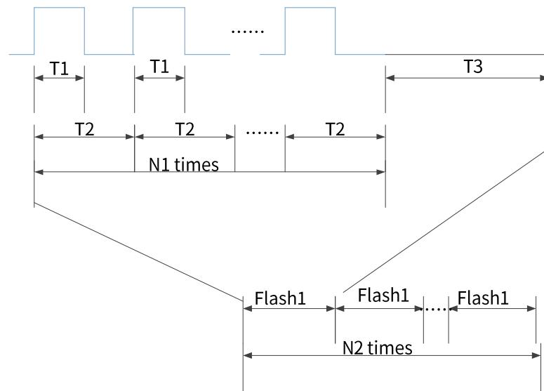
Figure 27. LED Breathing Light Setting Diagram
