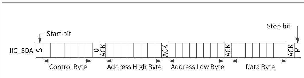
Figure 7.I<sup>2</sup>C Page Write Format
