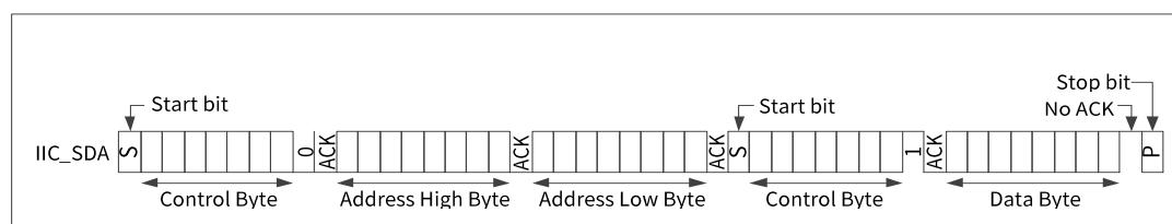
Figure 10. I<sup>2</sup>C Sequential Read Format
