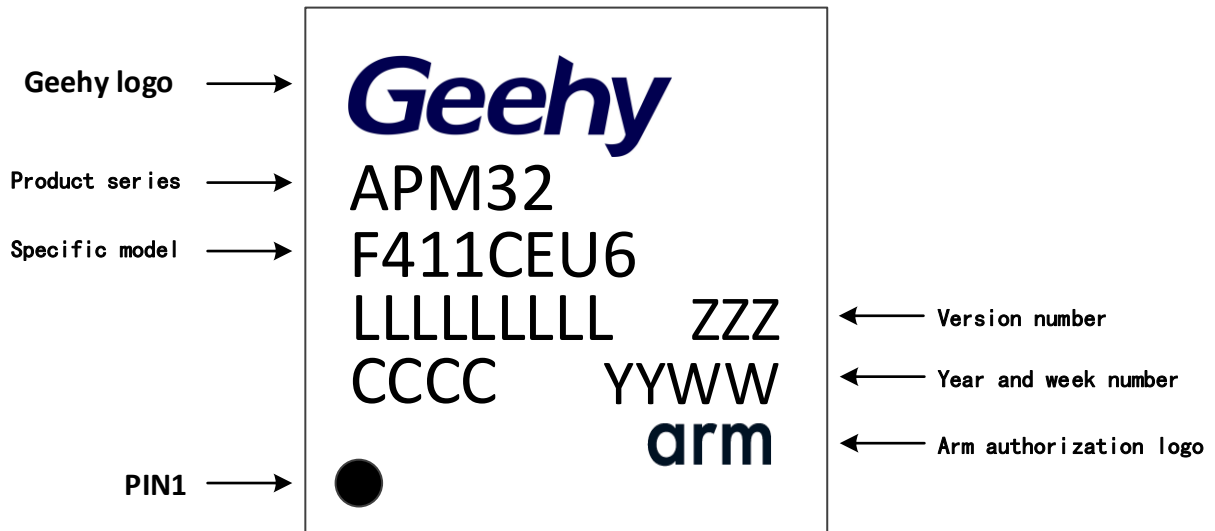
Figure 28 QFN448 - 48 Pins, 10 x 10mm Diagram
