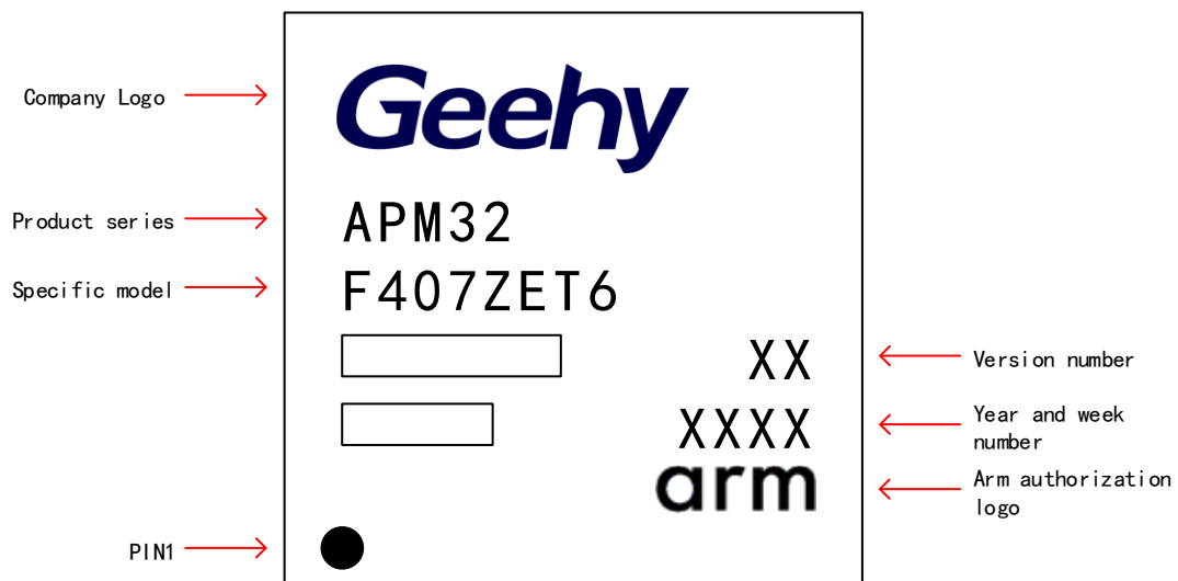
Figure 22 LQFP144 -144 Pins, 20 x20mm Schematic Diagram
