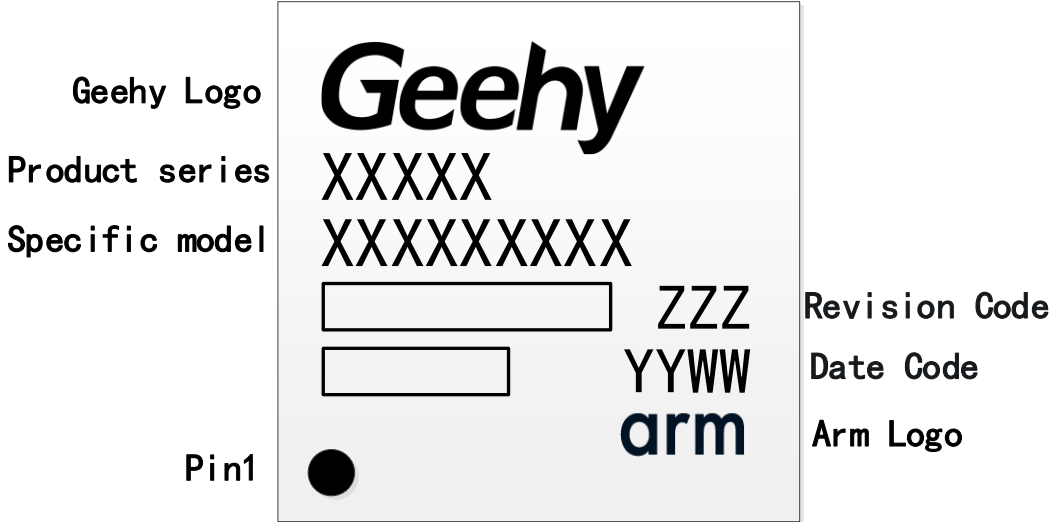
Figure 16 Product Silkscreen Diagram
